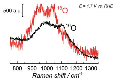
Fig. 3 SER spectra of NiOOH in the wavenumber region 800–1350 cm<sup>-1</sup>. The spectra were obtained at 1.7 V vs. RHE in Na<sup>16</sup>OH 0.1 M. The electrolyte was prepared with H<sub>2</sub><sup>16</sup>O and H<sub>2</sub><sup>18</sup>O.
