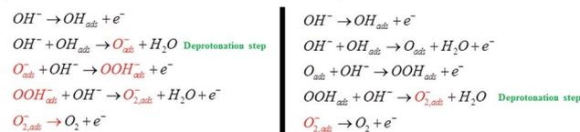
**Scheme 3** Comparison between the classical OER mechanism via concerted OH<sup>-</sup>/e<sup>-</sup> transfer and the decoupled mechanisms via decomposition of the negatively charged superoxo (O<sub>2</sub><sup>-</sup>) adsorbate generated by hydroxide-mediated deprotonation steps. The charges on the surface intermediates labeled in red should not be considered absolute, but as differential charges with respect to the surface species from which they are formed.
