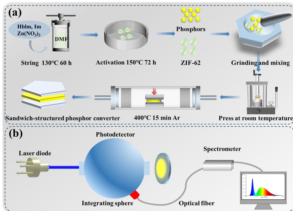
Fig. 1 (a) Fabrication procedure of the sandwich-structured LSN-in-ZIF-62 glass converter. (b) Schematics of the optical property measurement for the LSN-in-ZIF-62 glass converters under laser excitation.
