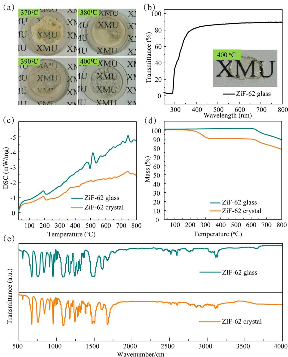
**Fig. 3** (a) Photographs of the ZIF-62 glasses sintered at different temperatures. (b) Transmittance spectrum of the ZIF-62 glass sintered at 400 °C. (c) DSC curves of the ZIF-62 crystal and ZIF-62 glass. (d) TG curves of the ZIF-62 crystal and ZIF-62 glass. (e) Infrared spectra of the ZIF-62 crystal and ZIF-62 glass.
