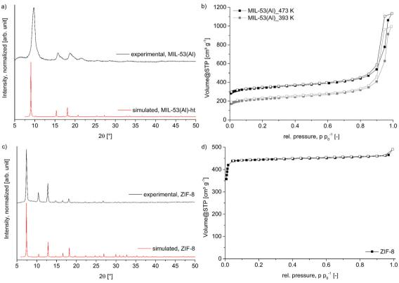
Fig. 3 a) PXRD pattern of synthesized MIL-53(AI) compared to the simulated pattern of the ht-form (CSD-Refcode: SABVUN01, ref. 57). b) Nitrogen-sorption isotherms of MIL-53(Al) after degassing at 393 K and 473 K. c) PXRD pattern of synthesized ZIF-8 compared to the simulated pattern (CSD-Refcode: FAWCEN, ref. 61). d) Nitrogen-sorption isotherm of ZIF-8. For the nitrogen-sorption isotherms the filled symbols represent the adsorption branch, while the empty symbols represent the desorption branch.
