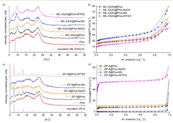
Fig. 4 a) and c) PXRD patterns of MIL-53(Al) and ZIF-8@wood composite materials. Simulated patterns were obtained from the crystal structures of MIL-53(AI) (CSD-Refcode: SABVUN01)<sup>57</sup> and ZIF-8 (CSD-Refcode: FAWCEN).<sup>61</sup> b) and d) Nitrogen-sorption isotherms (at 77 K) of MIL-53(AI) and ZIF-8@wood composite materials. For nitrogen-sorption isotherms, the filled symbols represent the adsorption branch, while the empty symbols represent the desorption branch.
