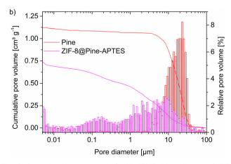
Fig. 6 Pore-size histograms of a) MIL-53(AI)@Pine-MA and b) ZIF-8@Pine-APTES from mercury intrusion porosimetry (MIP). For comparison, pristine Pine wood is shown in both histograms. The cumulative pore volume (scale at left) is given by the curves.
