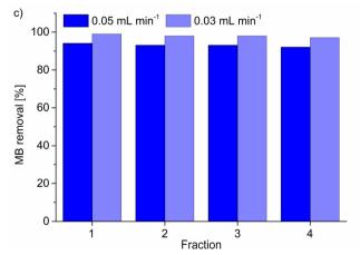
Fig. 8 a) Custom-made filtration capsule used to mount the MOF@wood composite for continuous filtration/catalysis. b) Setup for the continuous filtration/catalysis using a syringe pump and the custom-made filtration capsule. c) Results of the continuous filtration of MB from agueous solution using MIL-53(Al)@Pine-MA. One fraction is equal to 5 mL of MB solution pushed out of the syringe.
