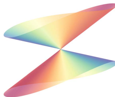
Fig. 9 Schematic illustration of a conical intersection for a two-dimensional system. The seam of the conical intersection consists of only one point. This point separates two adiabatic states from each other while the colors represent diabatic characters.
