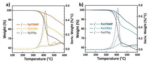
Fig. 4 TGA traces of the protonated precursor polymers in the TFSA<sup>−</sup> form and the AEMs in the Br<sup>−</sup> form recorded under N<sub>2</sub> atmosphere at a heating rate of 10 °C min<sup>-1</sup>: samples based on (a) pT and (b) mT, respectively
