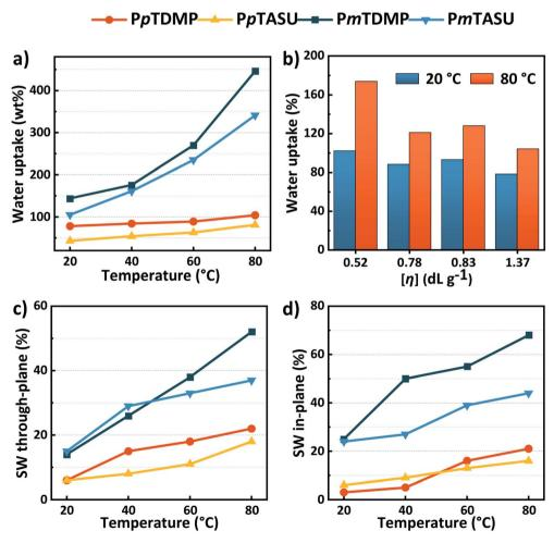
Fig. 5 Water uptake of AEMs based on pT and mT (a), and of AEMs based on PpTDMP samples with different [ $\eta$ ] values (b), as well as through- (c) and in-plane (d) swelling ratios of AEMs based on pT and mT. Data were measured between 20 and 80 °C on fully hydrated (immersed) samples in the OH<sup>-</sup> form.
