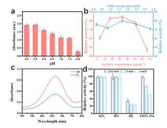
Fig. 4 Experimental condition optimization and mechanism study. The oxidase-like activity of Ag@MnO2 depended on: (a) pH and (b) concentration; (c) effect of dissolved oxygen; (d) the relative activity of the Ag@MnO2 catalytic system with ROS scavengers.
