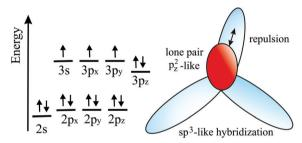
Fig. 19 Atomic orbitals of group V atoms with pyramidal sp<sup>3</sup>-like hybrids and a lone pair of  $p_z^2$ -like electrons
