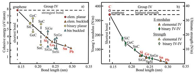
Fig. 13 (a) Plot of cohesive energy versus bond length of elemental and binary group IV monolayers in comparison to graphene. (b) Young's modulus and ultimate strength of elemental and binary group IV monolayers versus bond length in comparison to graphene.
