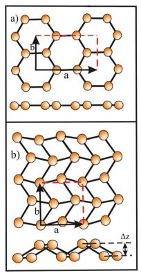
Fig. 6 (a) Honeycomb graphene-like lattice of gallenene obtained by cleaving bulk  $\alpha$ -Ga along the (100) direction after relaxation ( $a_{100}$ -Ga). (b) Distorted rhombic lattice of gallenene obtained by cleaving bulk  $\alpha$ -Ga along the (010) direction after relaxation (b<sub>010</sub>-Ga). The dashed rectangle and square show the unit cells
