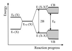
Fig. 14 Energy levels of hybridized s and p orbitals, reacting to molecular bonding and antibonding levels with level broadening and band formation of a monolaver.
