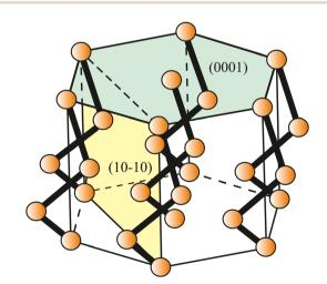
Fig. 24 Bulk structure of Se and Te with helical chains oriented in the zdirection assembled in a hexagonal arrangement. Two low-index crystal planes are indicated to illustrate possible cuts
