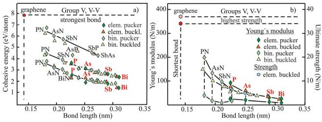
Fig. 20 (a) Cohesive energy *versus* bond length of elemental and binary group V monolayers. (b) Young's moduli and ultimate strengths *versus* bond length of elemental and binary group V monolayers.
