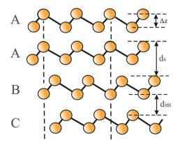
Fig. 15 The stacking orders AA, AB, and AC of bilayers of buckled hexagonal monolayers. This figure defines the buckling effect  $\Delta z$ , the interlayer spacing ds, and the distance between adjacent layers  $d_{\rm int}$
