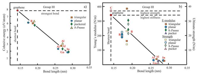
Fig. 7 (a) Plot of cohesive energy versus bond length for group III elemental monolayers. (b) Plot of Young's modulus and ultimate strength versus bond length of group III elemental monolayers.
