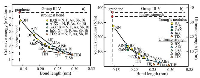
Fig. 17 (a) Cohesive energy versus bond length of group III-V monolayers in comparison to graphene. (b) Young's modulus and ultimate strength versus bond length of group III-V monolayers in comparison to graphene.
