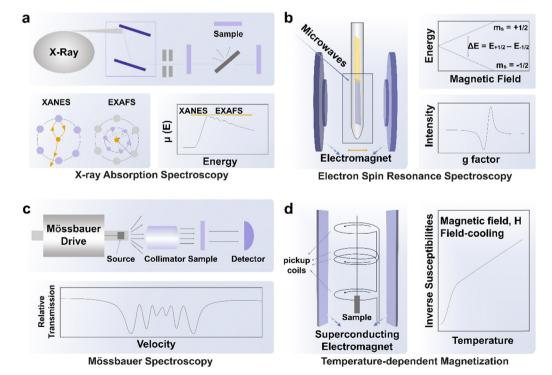
Fig. 3 Advanced characterization techniques for verification of spin state during electrocatalysis, including (a) XAS, (b) ESR, (c) Mössbauer spectroscopy, and (d) temperature-dependent magnetization
