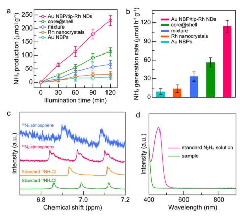
Fig. 4  $N_2$  photofixation under visible-NIR light illumination. (a)  $NH_3$  productions as a function of time for different catalysts. (b) Comparison of the  $NH_3$  production rates on different catalysts. (c) Isotope labelling experiments. (d) Detection of possible  $N_2H_4$  in the reaction system. The standard  $N_2H_4$  solution has an absorption peak at 455 nm.
