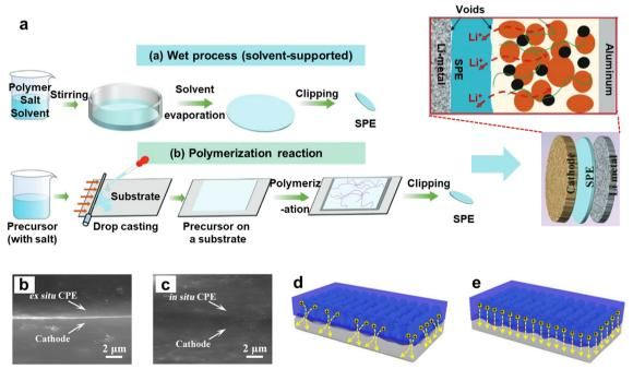
Fig. 6 (a) Ex situ polymerization route for preparing SPEs. Reproduced with permission.<sup>5</sup> Copyright 2023, John Wiley and Sons; (b) impact of in situ polymerization vs. ex situ polymerization; cross-sectional images of the interface between the ex situ CPE and cathode (b) vs. in situ CPE and cathode (c); schematic illustration of Li-ion transport at (d) the ex situ CPE||cathode interface and (e) in situ CPE||cathode interface. Reproduced with permission.<sup>78</sup> Copyright 2020.
