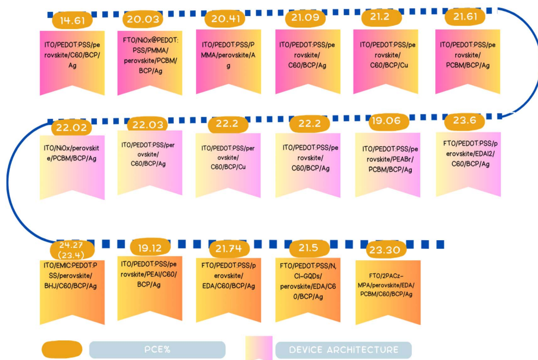
Fig. 11 Recent device performance of tin–lead mixed PSCs.
