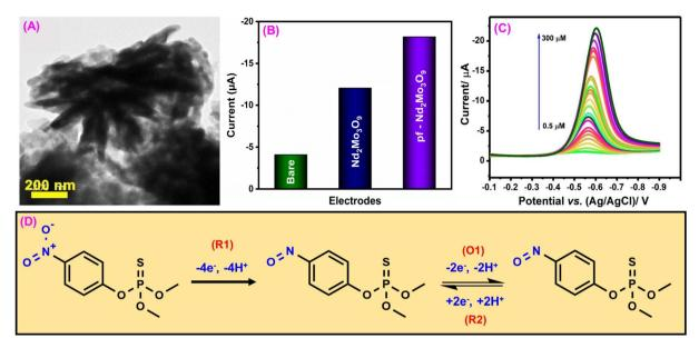
Fig. 2 (A) TEM image of pf-Nd<sub>2</sub>Mo<sub>3</sub>O<sub>9</sub>. (B) CV investigation of the bare GCE (green), Nd<sub>2</sub>Mo<sub>3</sub>O<sub>9</sub> (blue), and pf-Nd<sub>2</sub>Mo<sub>3</sub>O<sub>9</sub> (purple). (C) DPV signal of pf-Nd<sub>2</sub>Mo<sub>3</sub>O<sub>9</sub> for MPN detection. (D) Electrochemical detection mechanism of MPN<sup>103</sup> (modified). ((A and C) License number: 5542351439158).
