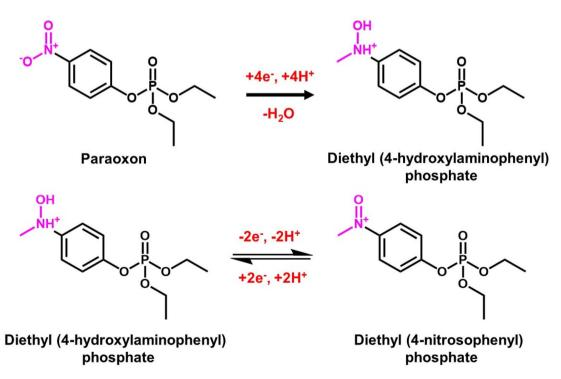
Fig. 6 The electrochemical oxidation mechanism of the paraoxon sensor.
