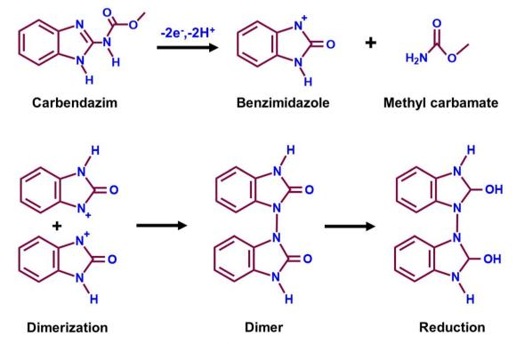
Fig. 4 The possible electrochemical detection mechanism of CRM.
