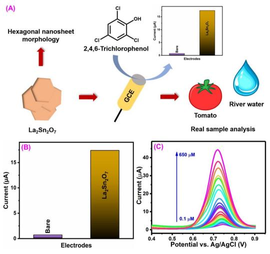
Fig. 8 (A) Schematic diagram for the synthesis of the  $La_2Sn_2O_7$  nanosheet and its electrochemical detection studies. (B) CV current response of the bare GCE and  $La_2Sn_2O_7/GCE$  towards TCL detection. (C) DPV response of  $La_2Sn_2O_7/GCE$  for detection of various concentrations of TCL<sup>124</sup> (modified). ((C) License number: 5570091012633).
