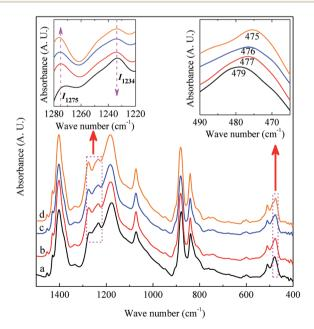
Fig. 6 FTIR spectra of electrospun membranes using 12 wt% of PVDF mixed with different  $V_{\text{NMP}}/V_{\text{acetone}}$  at 3/7, 4/6, 5/5, and 6/4 as labeled with 'a', 'b', 'c' and 'd', respectively. Insets are the magnification of frequency regions in 1220–1280 cm<sup>-1</sup> (left) and 465–490 cm<sup>-1</sup> (right). The arrows in the left inset indicate the direction of an increase in absorption
