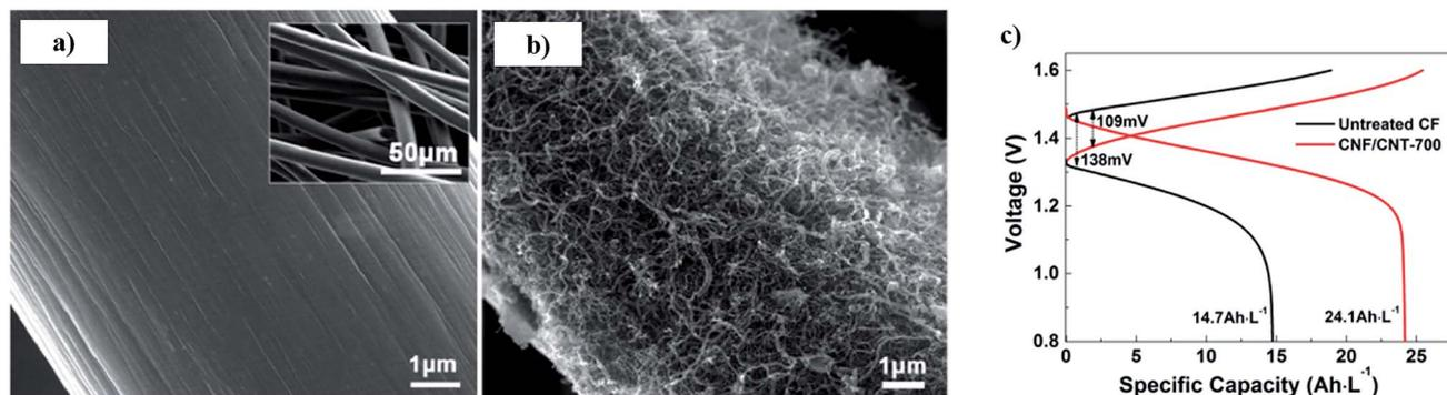
Fig. 11 SEM image of (a) untreated CF, (b) CNF/CNT grown CF surface. (c) Charge–discharge voltage profiles of VRFB employing untreated and CNF/CNT-T electrodes at 40 mA cm<sup>-2</sup>. Extracted from ref. 355.
