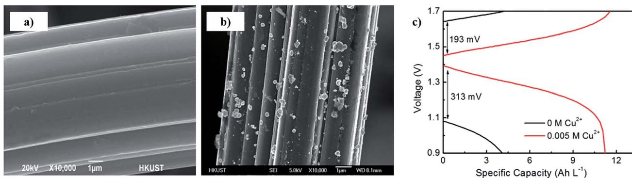
Fig. 12 SEM images of (a) original graphite felt and (b) the graphite felt decorated with copper nanoparticles. (c) Charge and discharge curves of VRFBs employing electrolytes containing different  $\text{Cu}^{2+}$  concentrations at  $300 \text{ mA cm}^{-2}$ . Extracted from ref. 361.
