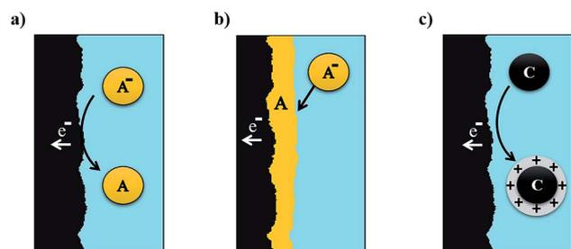
Fig. 3 Schematic representation of the electron transfer phenomena for the different types of RFB: all liquid (a), metal hybrid battery (b) and semi-solid (c).
