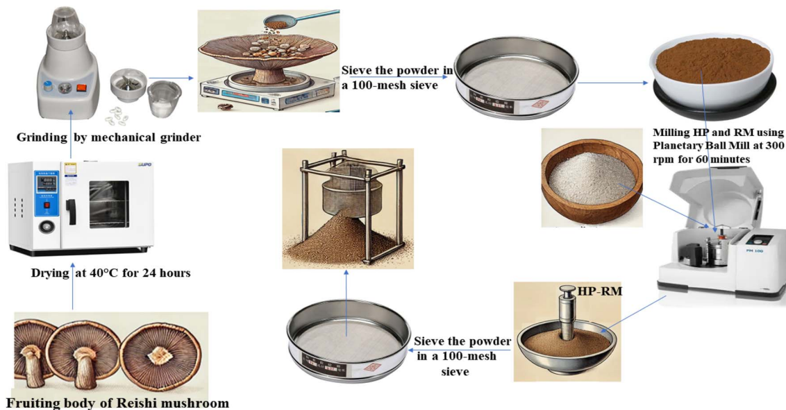
Scheme 1 Schematic representation of the experimental workflow for the preparation of the reishi mushroom fruiting body matrix and the loading of progesterone.
