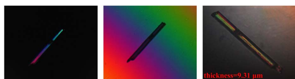
Fig. 5 Experimental birefringence at 546 nm for \text{Pb}_2(\text{SeO}_3)(\text{SiF}_6) .
