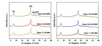
Fig. 1 PXRD patterns of nanosized Beta zeolites with varied Si/Al ratios.
