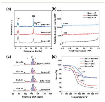
Fig. 6 Structures characterization of pure-silica Beta zeolites synthesized using different methods: (a) PXRD patterns, (b)  $N_2$  adsorption–desorption isotherms, (c)  $^{29}$ Si MAS NMR spectra, and (d) TG curves.
