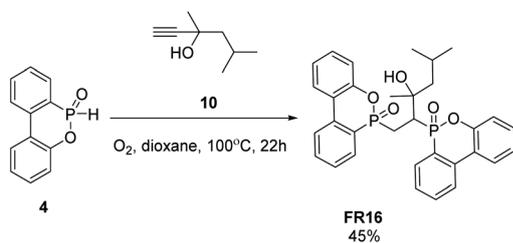
**Scheme 4** Synthesis process and structure of compound FR16. Reagents and conditions: **4** (3 eq.), **10** (1 eq.), O<sub>2</sub>, dioxane, 100 °C, 22 hours, 45%.
