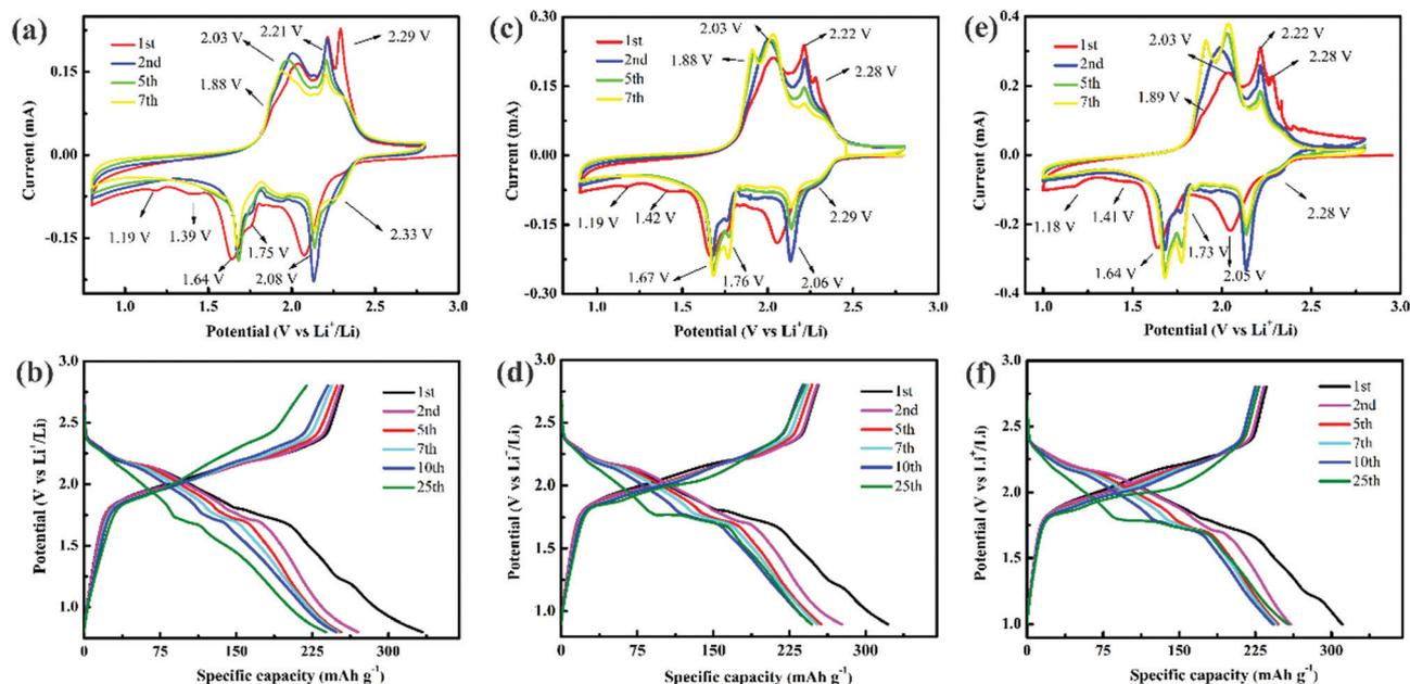
Fig. 2 CV curves at 0.1 mV s<sup>-1</sup> and discharge/charge curves at 0.1 mA cm<sup>-2</sup> of TiS<sub>2</sub> over (a and b) 0.8–2.8 V, (c and d) 0.9–2.8 V, and (e and f) 1.0–2.8 V.
