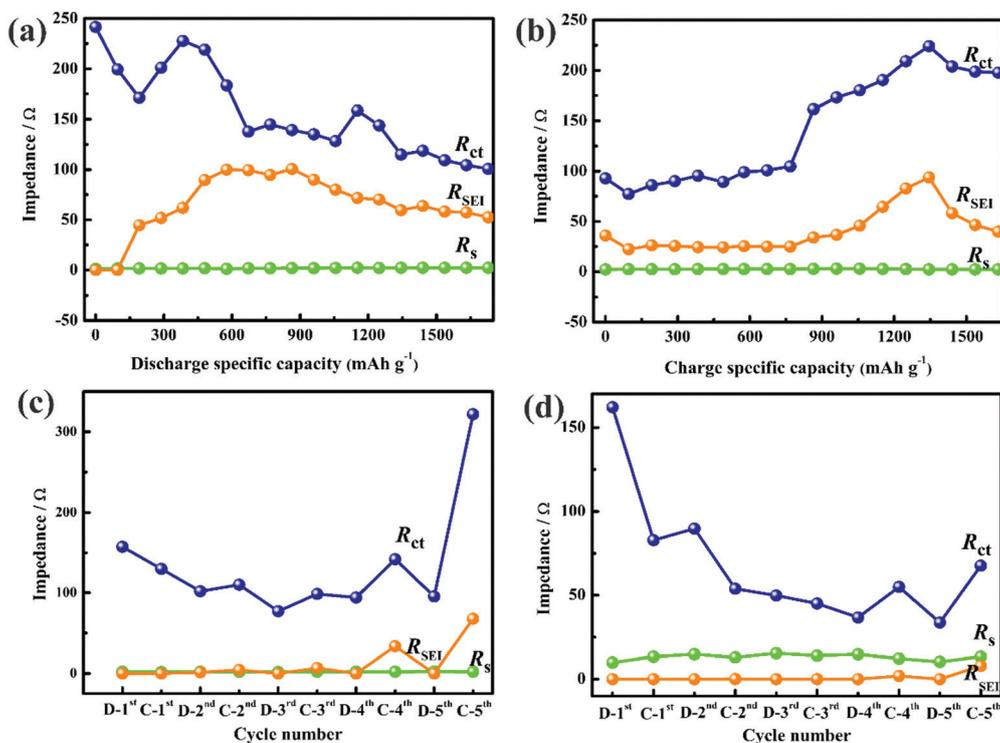
Fig. 3 Impedances of  $\text{TiS}_2$  at various (a) DODs and (b) DOCs during the first discharge/charge processes and at full states of discharge/charge for various cycles over (c) 0.8–2.8 V and (d) 0.9–2.8 V.
