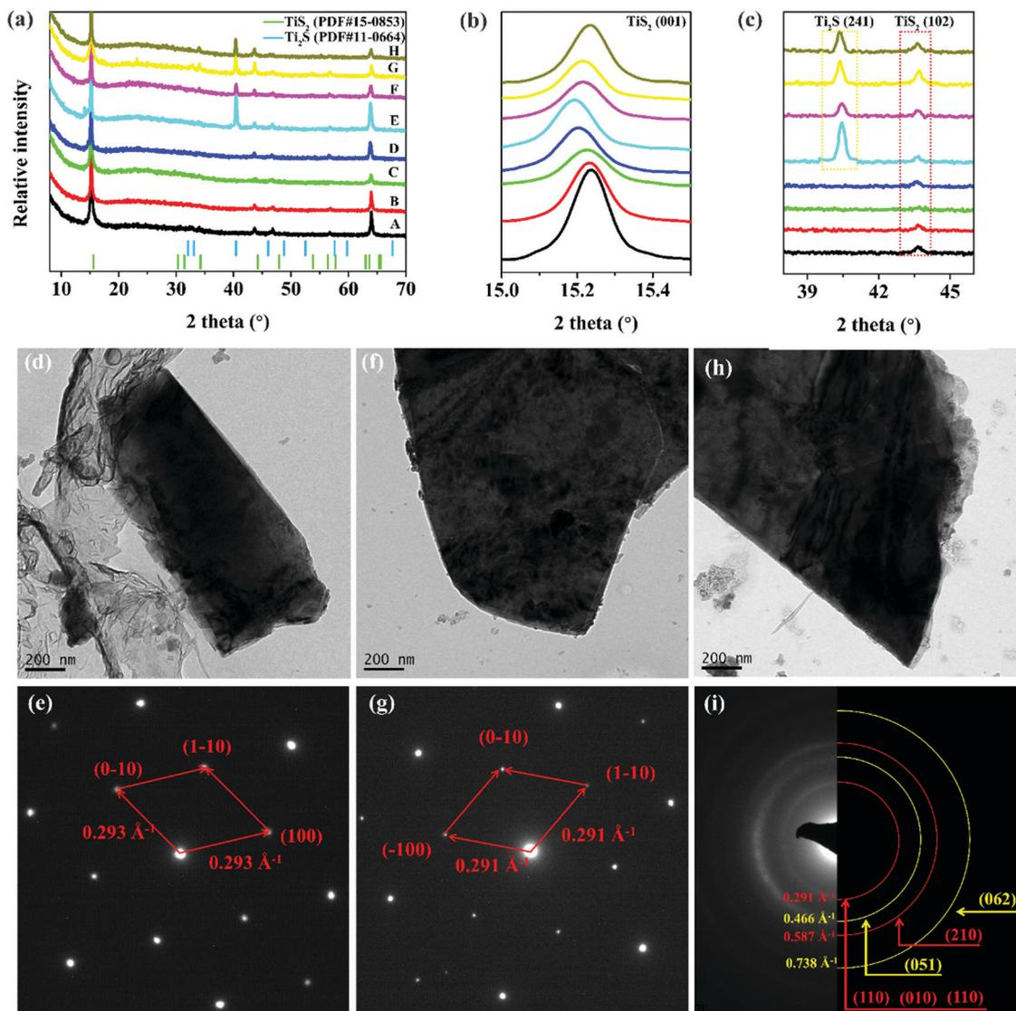
Fig. 5 (a–c) *Ex situ* XRD results at different states collected from Fig. S9 (ESI†). TEM and SAED images of  $\text{TiS}_2$  at (d and e) the initial state, and upon discharge to (f and g) 0.9 V and (h and i) 0.8 V.
