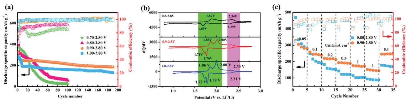
Fig. 1 (a) Cycling performance at 0.1 mA cm<sup>-2</sup>, (b) dQ/dV curves of the 25th discharge/charge curves at 0.1 mA cm<sup>-2</sup>, and (c) the rate performance of  $\text{TiS}_2$  across various electrochemical windows.
