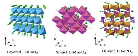
Fig. 2 Crystal structures of layered  $LiCoO_2$ , spinel  $LiMn_2O_4$  and olivine  $LiFePO_4$  cathode materials. Page Reproduced from open access article ref. 9 with permission MDPI, copyright 2014.
