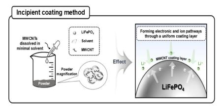
Fig. 12 Incipient coating of MWCNTs on LFP enhances electron and ion pathways.<sup>96</sup> Reproduced from ref. 96 with permission from the American Chemical Society, copyright 2025.
