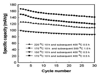
Fig. 5 Cycling stability of LiFePO<sub>4</sub> prepared at different temperatures.<sup>60</sup> This figure is adopted/reproduced/reprinted from ref. 60 with agreement from Elsevier, copyright 2007.
