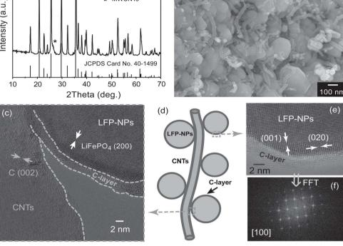
Fig. 17 (a) XRD pattern, (b) SEM, (c and e) HRTEM images, (d) schematic illustration of the generated LFP@C/CNT nanocomposite, and (f) the corresponding FFT from the HRTEM in (e). 122 Reproduced from ref. 122 with permission from John Wiley and Sons, copyright 2013.
