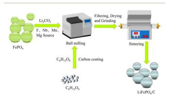
Fig. 15 Schematic representation of the carbothermal reduction process paired with a combined bulk phase doping approach to prepare LFP/C cathode materials. Reproduced from open access article ref. 98 with permission MDPI,copyright 2024.
