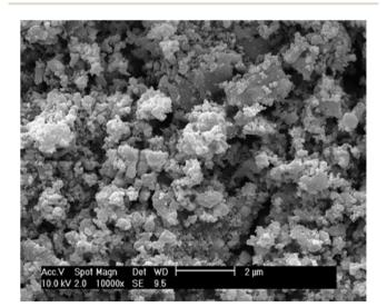
Fig. 7 SEM Analysis of LiFePO<sub>4</sub> particles synthesized by microwave heating for 4 minutes.<sup>64</sup> This figure is adopted/reproduced/reprinted from ref. 64 with permission from Elsevier, copyright 2003.
