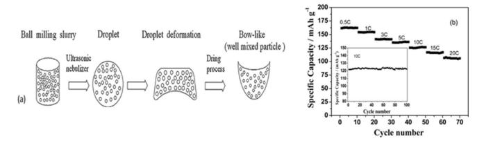
Fig. 8 (a) Formation scheme of the mesoporous bowl-like LiFePO<sub>4</sub>/C morphology and (b) its discharge profiles and rate capability at different current densities.<sup>66</sup> This figure being adopted/reproduced/reprinted from ref. 66 with permission from Elsevier, copyright 2003.
