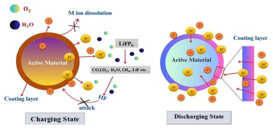
Fig. 3 Effect of surface coating on cathode materials in suppressing side reactions and enhancing structural stability.
