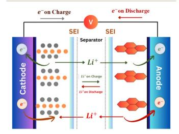
Fig. 1 Schematic of working principle of lithium ion battery during charge and discharge.
