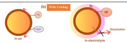
Fig. 10 Schematic illustration of cathode behavior with (b) and without carbon coating (a).
