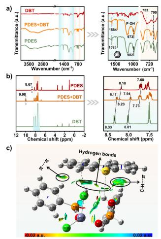
Fig. 5 (a) FT-IR and (b) <sup>1</sup>H NMR spectra of the product obtained from the reaction between the PDES and DBT. (c) Gradient isosurfaces (s = 0.35 a.u.) for the optimized structure of PDES-1-DBT-1. The surface is colored on a red-green-blue scale, according to the value of  $sin(\lambda)\rho$ , ranging from -0.02 to 0.02 a.u.
