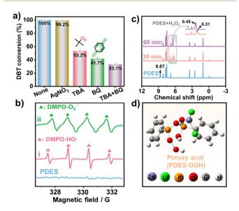
**Fig. 6** Reaction mechanism for the catalytic oxidation process. (a) Selective quenching experiments and (b) ESR spectroscopy for the identification of reactive radicals; i and ii: PDES reacts with  $H_2O_2$  for 10 min in deionized water and methanol as solvents. (c)  $^1H$  NMR spectra of the reaction between the PDES and  $H_2O_2$  for 30 min and 60 min. (d) Possible structure of peroxy acid (PDES-OOH).
