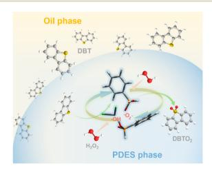
Scheme 1 ECODS mechanism using the bifunctional PDES ZnCl<sub>2</sub>/2PIA.
