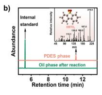
Fig. 4 (a) FT-IR spectra of the oxidation product. (b) GC-MS spectra of the main compounds in the reacted oil phase and PDES catalyst phase. Reaction conditions: m (PDES) = 1.0 g, V (model fuel containing DBT, 200 mg kg<sup>-1</sup>) = 5 mL, T = 45 °C, and O/S = 3.
