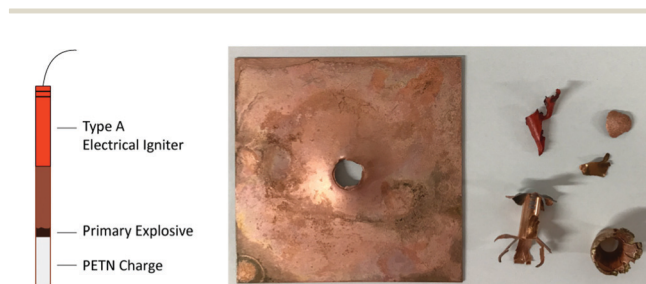
Fig. 21 Test setup for PETN Ignition experiments shown without the copper witness plate (left) and positive initiation experiment of compound 5a (right).
