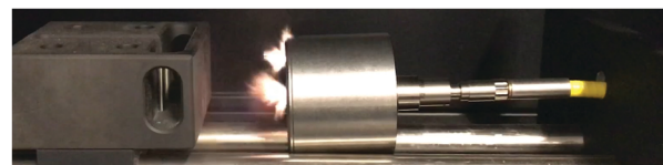
Fig. 22 Detonation of complex 9 during laser ignition experiments.
