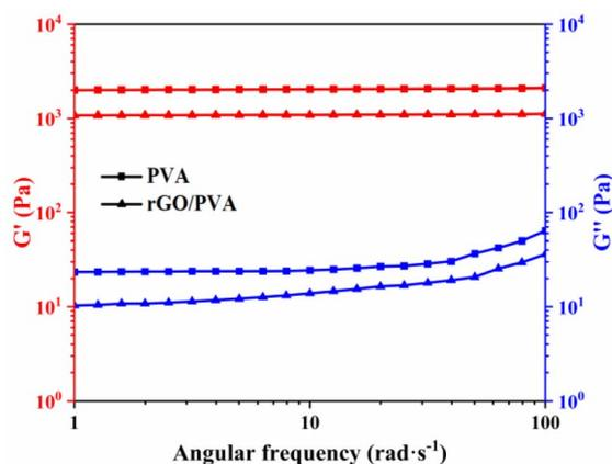
Fig. 9 Dynamic mechanical analysis of the energy storage modulus ( $G'$ ) and loss modulus ( $G''$ ) of the hydrogel.
