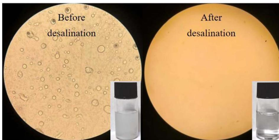
Fig. 16 Microscope images of oily seawater before and after desalination (insets are digital photographs).
