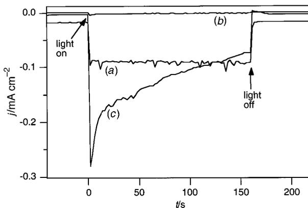
Fig. 1 Current density at -0.4 V measured on a 0.5 μm thick Cu<sub>2</sub>O electrode illuminated with 350 nm (5 × 10<sup>15</sup> s<sup>-1</sup> cm<sup>-2</sup>) in 0.5 M Na<sub>2</sub>SO<sub>4</sub> solution: (a) bubbled with air, (b) bubbled with Ar and (c) bubbled with Ar and with 40 mM MV<sup>2+</sup> added to the solution.
