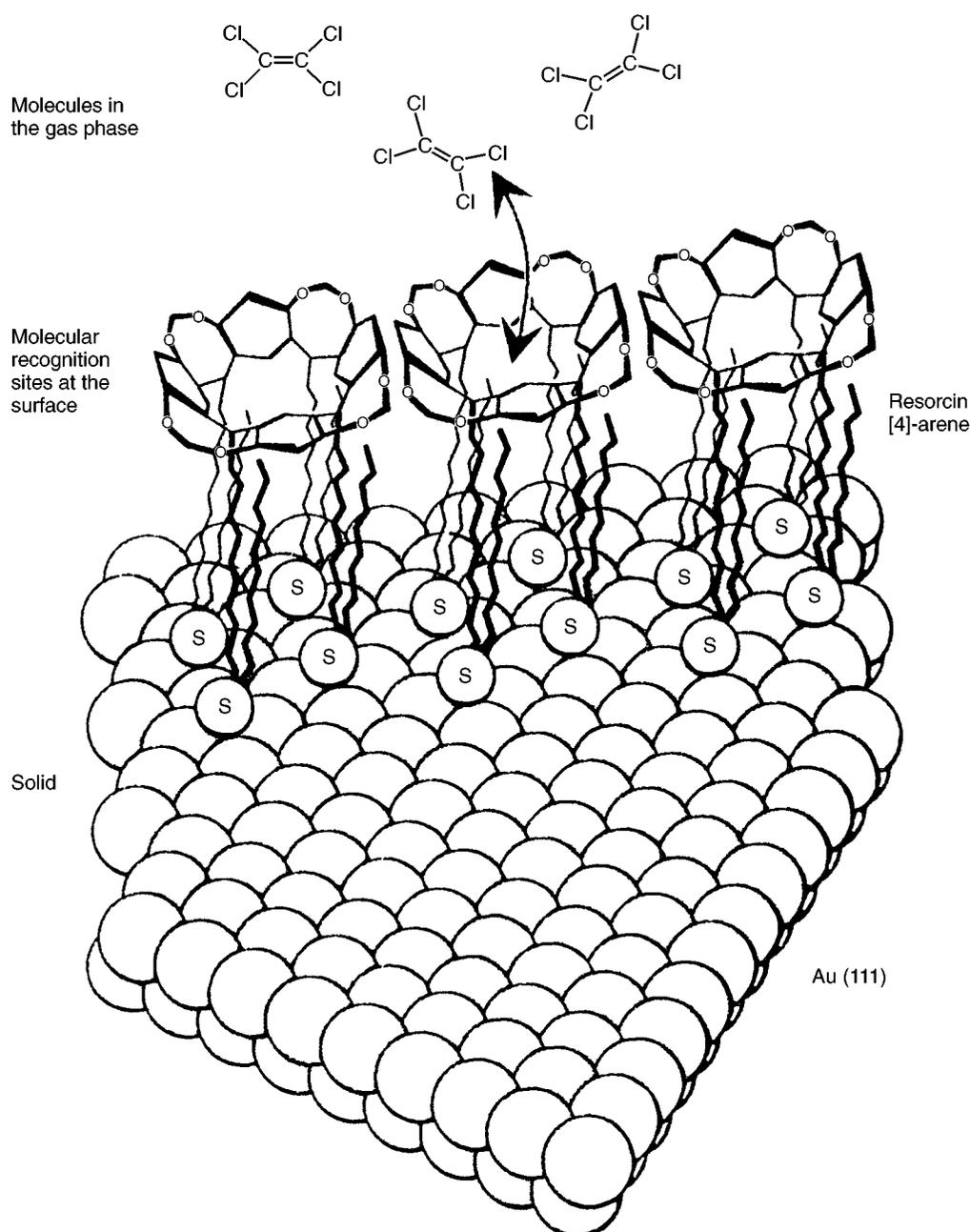
**Fig. 4** Schematic representation of the molecular structure and interaction of a self-assembled monolayer of resorcin[4]arenes on an Au(111) surface with perchloroethylene molecules from the gas phase.<sup>96</sup> (With kind permission from the American Association for the Advancement of Science).
