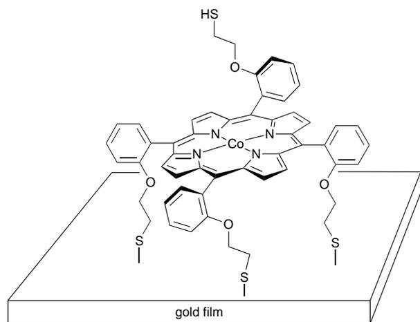
Fig. 3 Schematic illustration of the most probable average surface structure of tetra-thiolated cobalt porphyrin.<sup>69</sup> (With kind permission from the American Chemical Society.)
