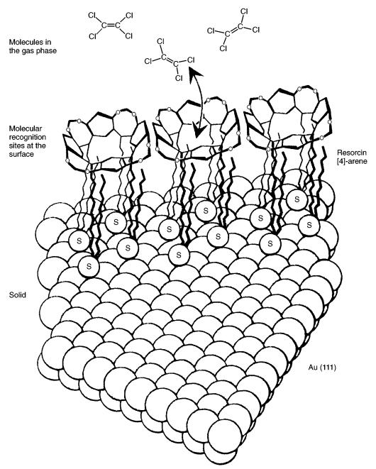
Fig. 4 Schematic representation of the molecular structure and interaction of a self-assembled monolayer of resorcin[4] arenes on an Au(111) surface with perchloroethylene molecules from the gas phase. 96 (With kind permission from the American Association for the Advancement of Science).
