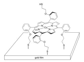
**Fig. 3** Schematic illustration of the most probable average surface structure of tetra-thiolated cobalt porphyrin.<sup>69</sup> (With kind permission from the American Chemical Society.)
