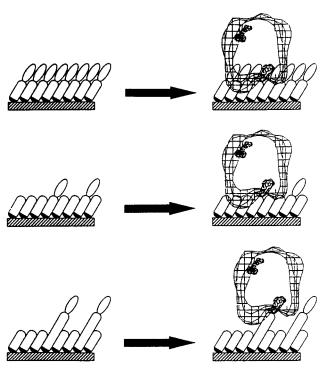
**Fig. 2** Schematic representation of a SAM of thiols and the binding of streptavidin to them. (Top) A pure monolayer. Binding of streptavidin is severely sterically hindered. (Center) A monolayer of a mixture of thiols with the same length of the alkane moiety. There still is steric hindrance. (Bottom) Addition of a spacer allows binding without steric hindrance. <sup>83</sup> (With kind permission from Elsevier Science Ltd.)
