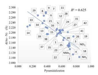
Fig. 4 Pyramidalization vs. Au-N distance (in Å) correlation.
