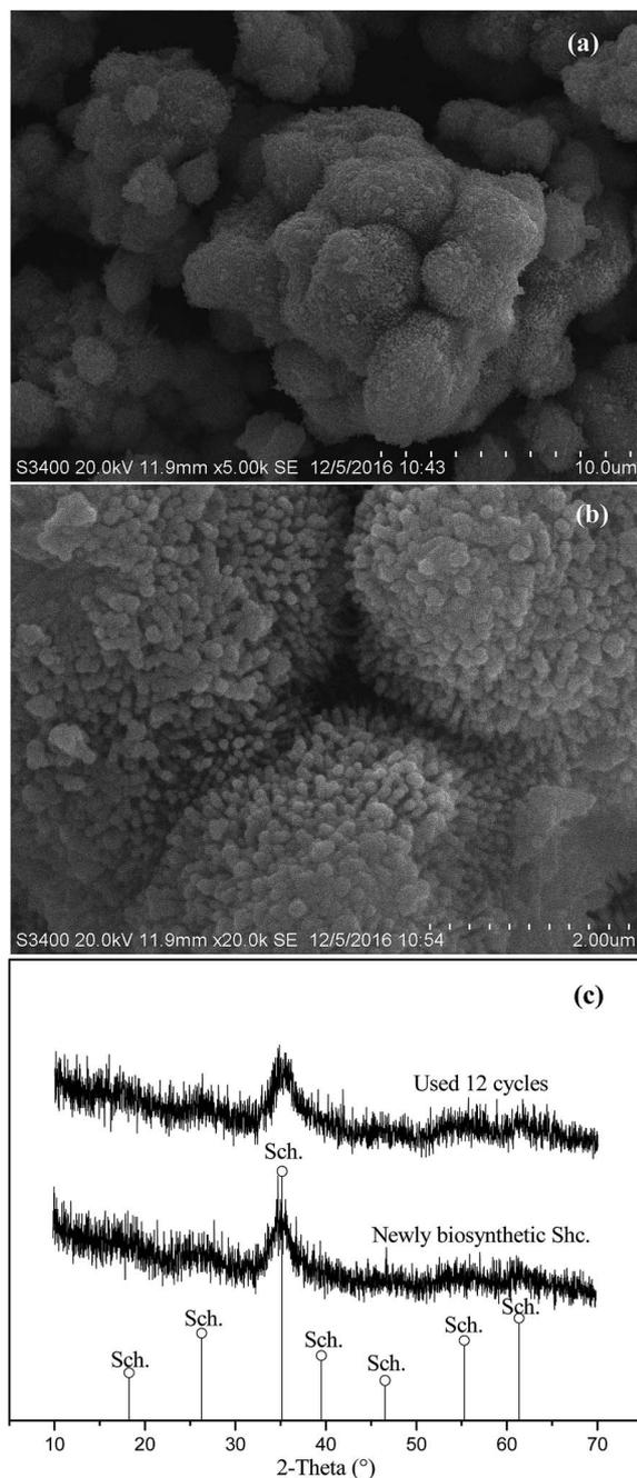
Fig. 1 SEM images of the biosynthetic schwertmannite particles:  $\times 2000$  (a) and  $\times 20\,000$  (b), and XRD (c) analyses of newly biosynthesized schwertmannite and the schwertmannite after being used for 12 cycles. Experimental conditions were  $[\text{phenanthrene}]_0 = 1 \text{ mg L}^{-1}$ ,  $[\text{schwertmannite}]_0 = 1 \text{ g L}^{-1}$ ,  $[\text{H}_2\text{O}_2]_0 = 200 \text{ mg L}^{-1}$ , solution initial pH = 3.0, and reaction time of 12 h in each cycle.
