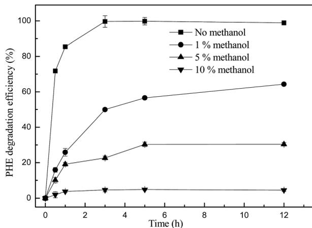
Fig. 4 Effect of methanol addition on the degradation of phenanthrene with working volume of 10 mL. Experimental conditions were  $[\text{phenanthrene}]_0 = 1 \text{ mg L}^{-1}$ ,  $[\text{schwermannite}]_0 = 1 \text{ g L}^{-1}$ ,  $[\text{H}_2\text{O}_2]_0 = 200 \text{ mg L}^{-1}$ , and solution initial pH = 3.0.
