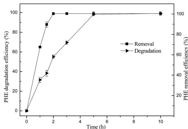
Fig. 7 Changes of phenanthrene degradation efficiency and its removal efficiency during the catalytic degradation with working volume of 10 mL. Experimental conditions were  $[\text{phenanthrene}]_0 = 1 \text{ mg L}^{-1}$ ,  $[\text{schwertmannite}]_0 = 1 \text{ g L}^{-1}$ ,  $[\text{H}_2\text{O}_2]_0 = 200 \text{ mg L}^{-1}$ , and solution initial pH = 3.0.
