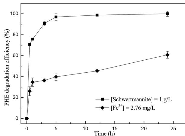
Fig. 6 Change of phenanthrene degradation efficiency during the degradation catalyzed by  $1 \text{ g L}^{-1}$  schwertmannite or  $2.7 \text{ mg L}^{-1}$   $\text{Fe}^{3+}$ , with working volume of  $10 \text{ mL}$ . Experimental conditions:  $[\text{phenanthrene}]_0 = 1 \text{ mg L}^{-1}$ ,  $[\text{H}_2\text{O}_2]_0 = 200 \text{ mg L}^{-1}$ , and solution initial pH = 3.0.
