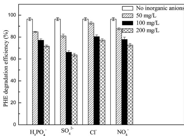
Fig. 10 Effect of inorganic anions ( $\text{H}_2\text{PO}_4^-$ ,  $\text{SO}_4^{2-}$ ,  $\text{Cl}^-$ ,  $\text{NO}_3^-$ ) on the degradation of phenanthrene with working volume of 10 mL. Experimental conditions were  $[\text{phenanthrene}]_0 = 1 \text{ mg L}^{-1}$ ,  $[\text{schwertmannite}]_0 = 1 \text{ g L}^{-1}$ ,  $[\text{H}_2\text{O}_2]_0 = 200 \text{ mg L}^{-1}$ , and solution initial  $\text{pH} = 3.0$ .
