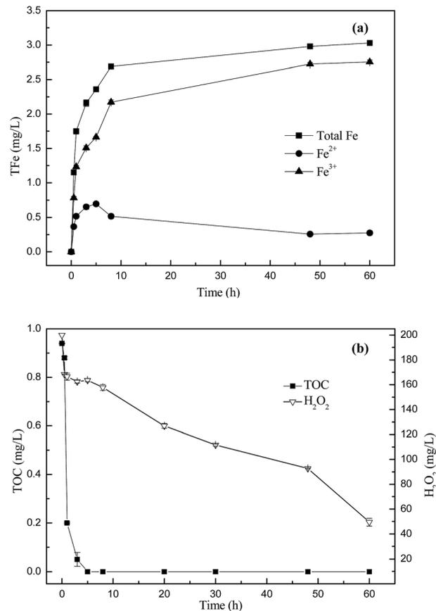
Fig. 5 Changes of total Fe (TFe),  $\text{Fe}^{2+}$  and  $\text{Fe}^{3+}$  concentration (a),  $\text{H}_2\text{O}_2$  concentration and TOC content (b) in the solution during the degradation of  $1 \text{ mg L}^{-1}$  phenanthrene catalyzed by  $1 \text{ g L}^{-1}$  of schwertmannite and  $200 \text{ mg L}^{-1}$   $\text{H}_2\text{O}_2$  at pH 3.0.
