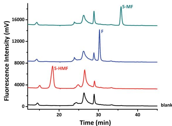
Fig. 4 Respective HPLC analysis of **F**, **5-MF**, **5-HMF** derivatization mixtures, compared with corresponding HPLC analysis of compound **1a** as a sample blank.
