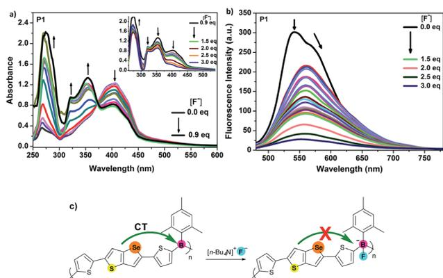
Fig. 3 (a) Absorption spectra and (b) emission spectra ( $\lambda_{exc} = 470$  nm) of **P1** ( $1 \times 10^{-4}$  M based on boron sites) in THF in the presence of various amounts of TBAF. (c) Pictorial view of interruption of charge transfer (CT) by fluoride binding.
