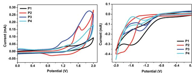
Fig. 2 Cyclic voltammograms of the polymers **P1–P4** on glassy carbon disk electrode in acetonitrile, 0.1 M Bu<sub>4</sub>NPF<sub>6</sub>, 100 mV s<sup>−1</sup> scan rate, vs. Fc/Fc<sup>+</sup>.
