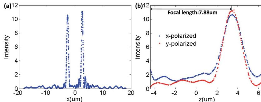
Fig. 6 (a) The electric field intensity along the  $x$ -axis and (b) the  $z$ -axis at the focal plane.
