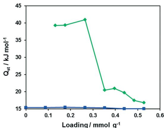
Fig. 10 Dependencies of the isosteric heats of O<sub>2</sub> (blue) and CO (green) adsorption on the loading for CFA-9.
