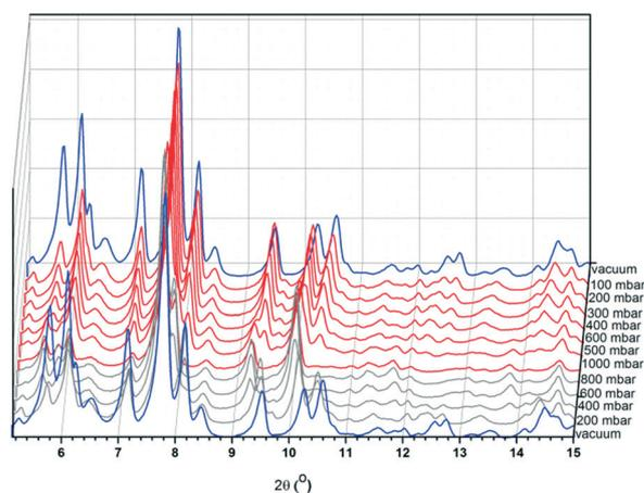
Fig. 9 XRPD plots of CFA-9 measured at -78.5 °C under vacuum (blue lines) and under increasing CO<sub>2</sub> pressure (red lines) and decreasing CO<sub>2</sub> pressure (grey lines).
