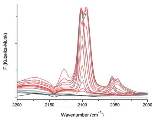
Fig. 11 *In situ* DRIFT spectra of CFA-9 recorded in 20 °C steps upon cooling from 100 °C to -100 °C under a CO atmosphere (red lines) and subsequent heating from -100 °C to 100 °C under an Ar atmosphere (gray lines). The DRIFT spectrum of KBr at -60 °C under a CO atmosphere (black line).
