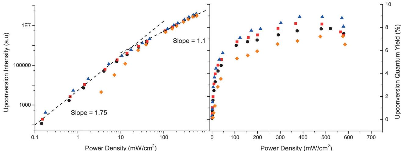
Fig. 7 Left: A double logarithmic plot of integrated upconverted emission dependence on excitation power density (532 nm) of solutions containing PtOEP, 15  $\mu\text{M}$  and 0.5 mM annihilator. Right: Upconverted emission quantum yield ( $\Phi_{\text{UC}}$ ) as a function of excitation power density of the same solutions. 1 (●), 3 (■), 4 (▲) and 5 (◆).
