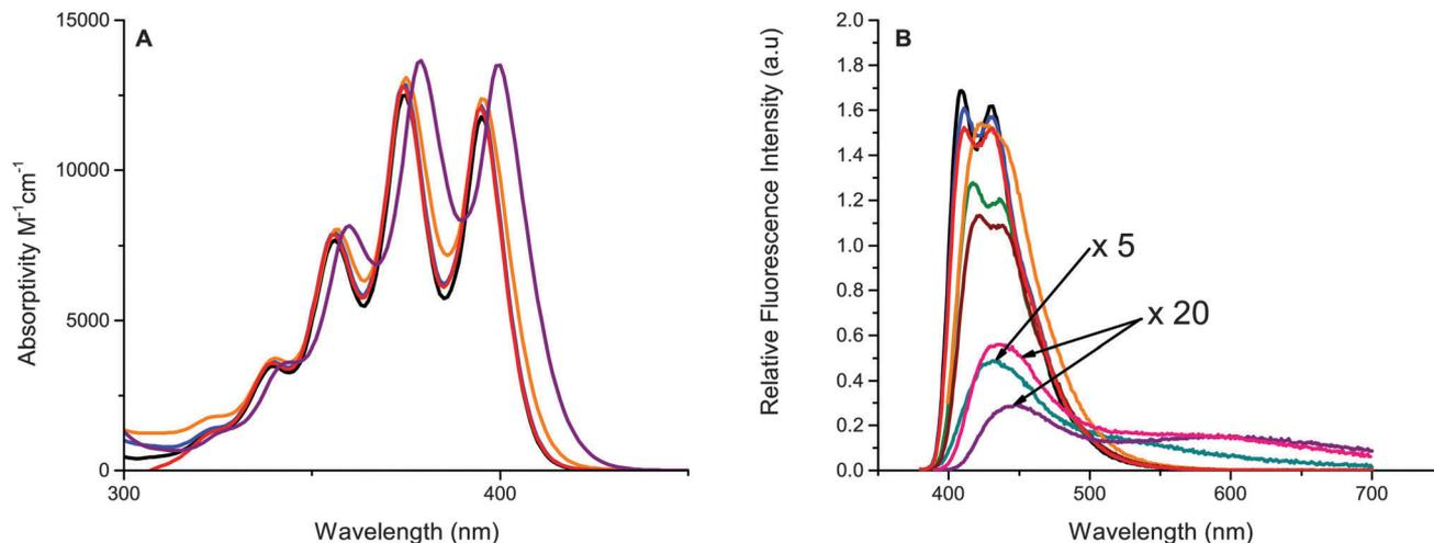
Fig. 4 (A) Molar absorptivity of the representative compounds **1** (—), **3** (—), **4** (—), **5** (—), and **8** (—) and (B) relative fluorescence intensity of synthesized anthracene derivatives compared to **1** (—), **3** (—), **4** (—), **5** (—), **6** (—), **7** (—), **8** (—), **9** (—) and **10** (—); spectra are corrected for differences in absorbance at excitation wavelength.
