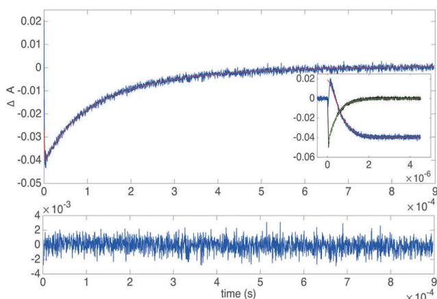
Fig. 6 Transient absorption measurements of **4** (1 mM) and PtOEP (3.4 μM) at 410 nm (annihilator decay, blue) and 650 nm (sensitizer decay, black) and the respective fits. The inset shows the first 5 μs. The bottom panel shows the residual of the fitted annihilator decay.
