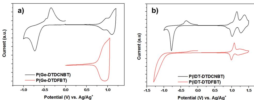
Fig. 3 Cyclic voltammograms of thin films of (a) P(Ge-DTDCNBT) and P(DTDFBT) (b) P(IDT-DTDCNBT) and P(IDT-DTDFBT) in acetonitrile- $[\text{n-Bu}_4\text{N}]\text{PF}_6$  solutions ( $0.1 \text{ M}$ ) at a scan rate of  $100 \text{ mV s}^{-1}$ .
