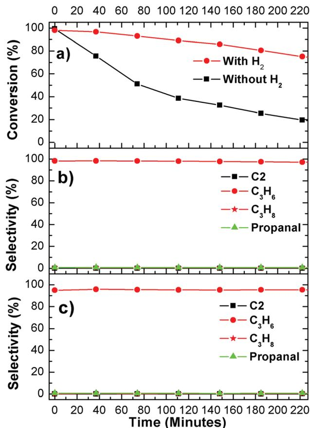
Fig. 6 Flow reactor results of propanol deoxygenation reactions at 653 K (reaction conditions:  $\text{H}_2$ -propanol = 10 : 1, catalyst 43.5 mg): (a) conversion; (b) selectivity with co-feed  $\text{H}_2$ ; and (c) selectivity without co-feed  $\text{H}_2$ .
