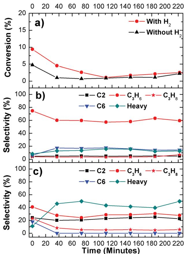
Fig. 7 Flow reactor results of propanol deoxygenation reactions at 653 K (reaction conditions:  $\text{H}_2$ -propanol = 10 : 1, catalyst 43.5 mg): (a) conversion; (b) selectivity with co-feed  $\text{H}_2$ ; and (c) selectivity without co-feed  $\text{H}_2$ .
