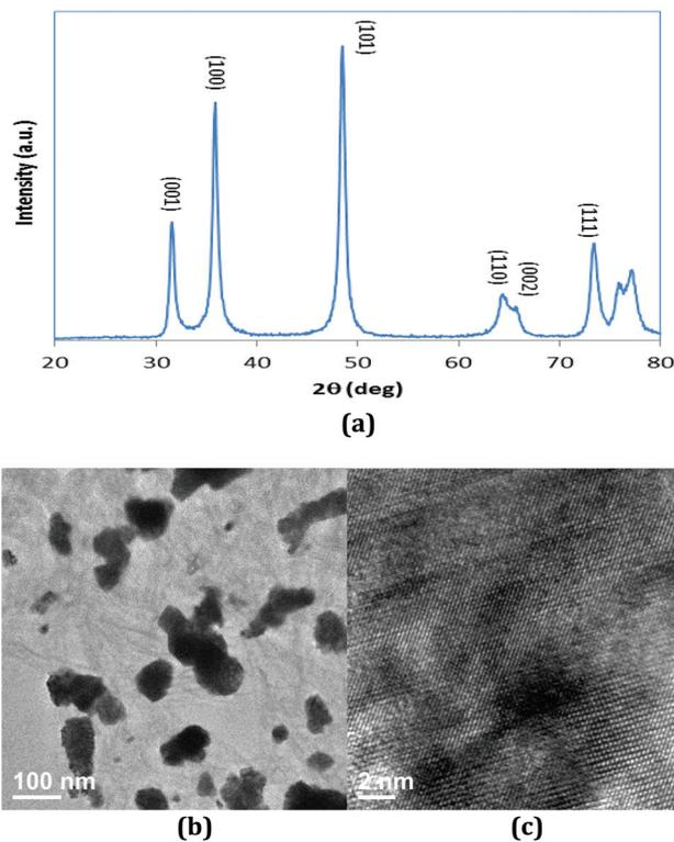
**Fig. 5** Characterizations of powder WC: (a) XRD; (b) TEM; (c) HRTEM.
