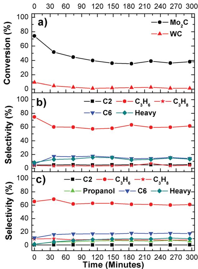
Fig. 8 Comparison of propanal with H<sub>2</sub> reactions on WC and Mo<sub>2</sub>C: (a) conversion; (b) selectivity over WC; and (c) selectivity over Mo<sub>2</sub>C.
