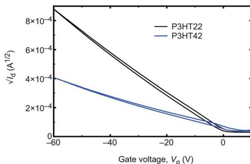
**Fig. 5** Transfer characteristics for samples with P3HT brushes on SiO<sub>2</sub> as gate insulators after annealing at 100 °C for 24 h ( $V_T = -0.3$  and 4.4 V for the P3HT22 and P3HT42 respectively). In these experiments,  $V_d = -60$  V.
