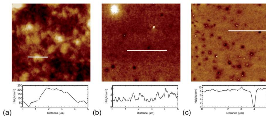
**Fig. 3** Scanning force microscopy images of P3HT layers: (a) P3HT17 unannealed spin-coated onto a silicon substrate; (b) P3HT17 annealed at 100 °C for 24 h; and (c) P3HT28 annealed at 100 °C for 24 h. 5 μm height scans are indicated for the region covered by the white line in each image.
