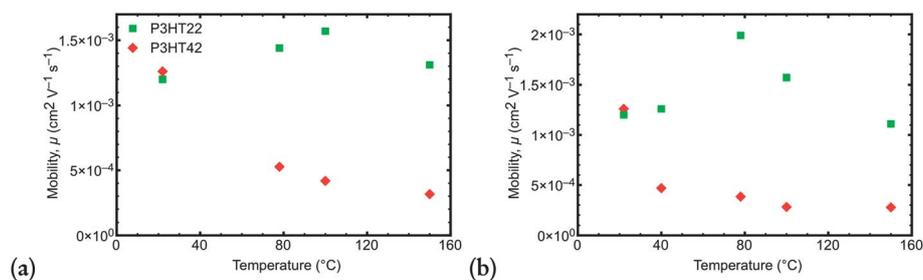
**Fig. 7** Saturated hole mobility data as a function of annealing temperature for 5 minutes annealing (a) and for 24 h annealing (b). The samples “annealed” at 22 °C are unannealed reference samples (a 700 nm spin coated PMMA layer rather than a brush); the temperature represents room temperature.
