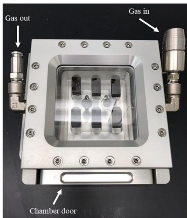
Figure 1. Sealed sample chamber used to maintain an inert atmosphere of either argon or helium during storage and measurements. The sample chamber has two gas connectors, an inlet, and an outlet that allow for gas to be flowed through the chamber.
