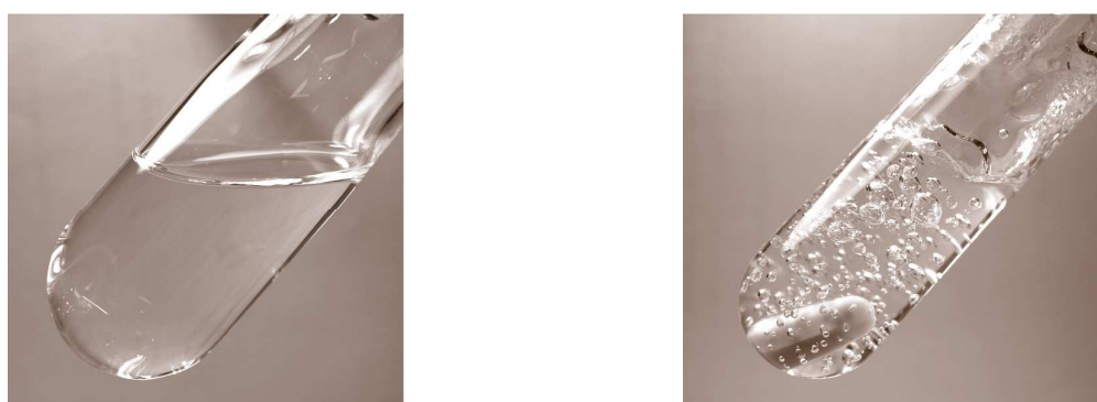
Fig. 1: Photographs of a \text{MgF}_2 sol (left) and \text{MgF}_2 gel with air bubbles (right)
