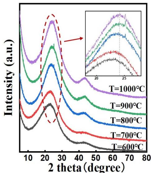
Fig. 1 XRD patterns of the various samples.
