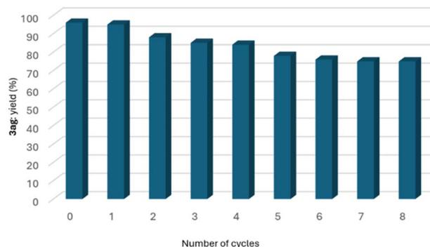
Fig. 1 Reusing of FeCl<sub>3</sub>·6H<sub>2</sub>O/Gly LADES in the synthesis of Chlodantane (**3ag**) from 2-adamantanol (**1o**) and *p*-chlorobenzotrile (**2d**).
