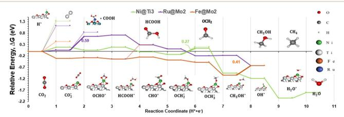
Fig. 7 Energy diagram for Ni@Ti<sub>3</sub>, Ru@Mo<sub>2</sub>, and Fe@Mo<sub>2</sub>. The diagram includes the pathways to methane ( $CH_4$ ) and methanol ( $CH_3OH$ ). On the bottom, the main intermediates are presented and match the curves above. On top, the final products, side products or intermediates are shown and match the thin curves below them, if applicable. The reaction coordinate number represents the number of PCET steps, except for adsorption and desorption steps.
