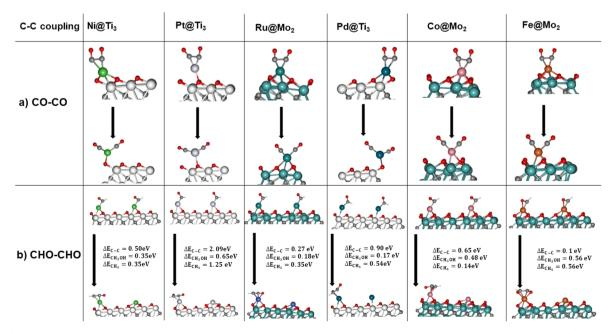
Fig. 6 (a) \*CO + \*CO coupling. The first image is before optimization while the bottom image is the optimized structure. (b) \*CHO + \*CHO coupling and the reaction energy comparatively to methanol and methane production.
