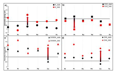
Fig. 5 Adsorption energies of: (a) H and (b) CO<sub>2</sub> on a slab and SAC, for the six chosen transition metals. Similarly, desorption energies of: (c) CH<sub>3</sub>OH and (d) CH<sub>4</sub>. Arrows show the biggest difference between the slab and SAC for each sub-figure.
