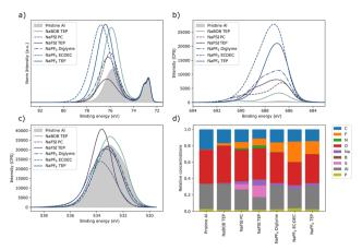
Fig. 4 XPS deconvolution results of the spectra shown in Fig. S6-S8 (ESI†). The spectra shown here are energy calibrated to the "bulk"-signal of aluminum Al2p positioned to 72.7 eV, (a) Al2p, (b) F1s, and (c) O1s core levels. The relative atomic concentrations are shown in (d), this estimation is based on the models in Fig. S6-S8 (ESI†). The spectra in (a) have been area normalized to the intensity that was believed to be caused by the pure aluminium ("bulk" aluminium).
