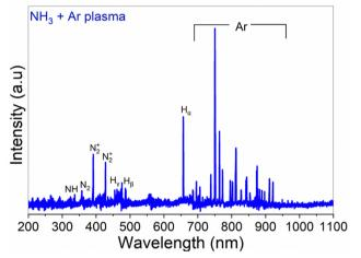
Fig. 3 Optical emission spectra for Ar and NH<sub>3</sub> + Ar plasmas at 2800 W over the wavelength range of 200-1100 nm showing the different reactive species available for reaction with TMA during the plasma process.
