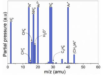
Fig. 4 A survey scan showing average intensities of all detected masses during 5 ALD cycles of the TMA-NH<sub>3</sub> process. No other species were detected beyond m/z 60
