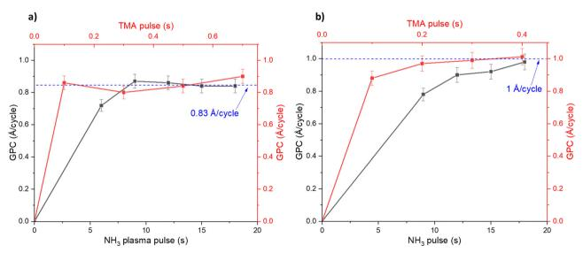
Fig. 1 Saturation curves for the plasma ALD (a) and thermal ALD (b) processes, showing the effect of the TMA pulse time and the (a)  $NH_3$  plasma time, or the  $NH_3$  pulse time (b) on the GPC in the ALD processes. The plasma process is studied at 300 °C and the thermal process at 350 °C.
