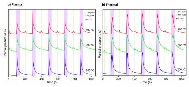
Fig. 5 Mass spectrometric time behaviour of detected  $CH_4^+$  (m/z = 16) during five AIN growth cycles from TMA and  $NH_3$  in both plasma (a) and thermal (b) processes at different temperatures. The pulse times were fixed at 0.2 s for TMA and 12 s for  $NH_3$  with 90 s purging in between. The graphs are expressed in arbitrary units and have been vertically shifted for visual clarity.
