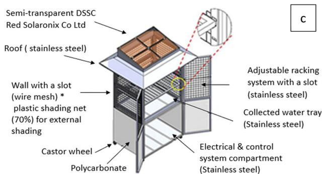
Fig. 12 (a) and (b) DSSM application in an Aquaponic greenhouse.<sup>17</sup> (c) The detailed construction drawings of PDMG prototype. Reproduced with permission ref. 233 Elsevier.
