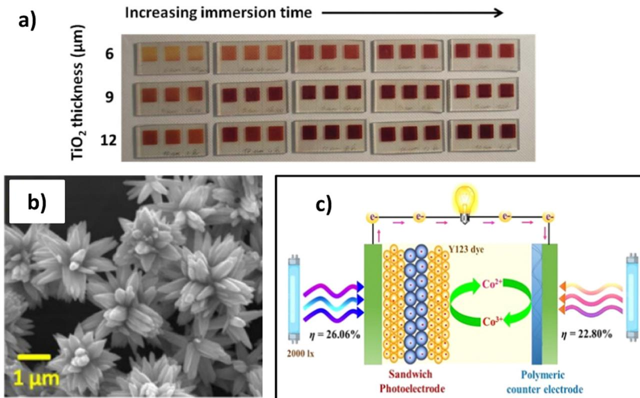
Fig. 8 (A) Comparison of fabricated WE with N719 dye considering the TiO<sub>2</sub> thickness and the immersion time. Reproduced and adapted from ref. 177. (B) SEM image of ZnO micro-flowers applied as SL from ref. 179 under Creative Commons BY-4.0 license (c) sandwich photoelectrode structure realized by ML-SL-ML from ref. 134 Copyright © 2022 American Chemical Society.
