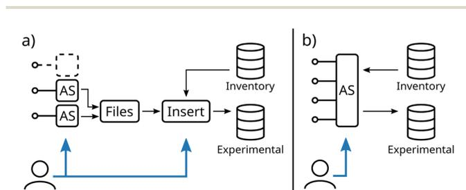
Fig. 3 Schematic communication between database and acquisition software (AS) controlling different measurement devices. Blue arrows indicate required user interaction. (a) Communication *via* exported data files (b) integrated database communication.
