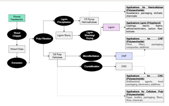
Fig. 1 Conceptual representation of the process flow for the extraction of wood derivatives (roughly based on the Fabiola process<sup>28–30</sup>) along with their respective applications. Additional details about other extraction processes may be obtained from the literature compiled in the ESI.†
