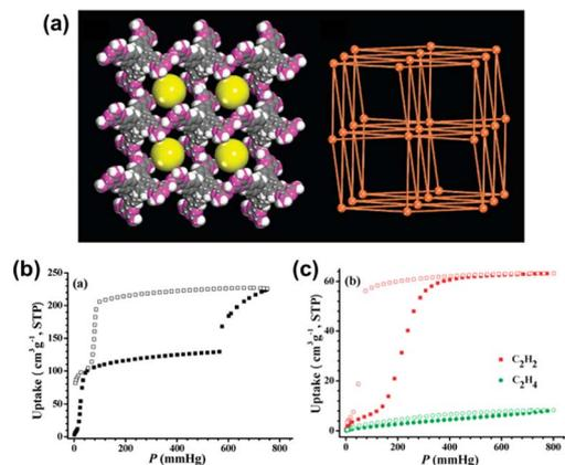
Fig. 4 (a) Single-crystal structure and topology of HOF-1; (b) CO<sub>2</sub> adsorption at 196 K; (c) C<sub>2</sub>H<sub>2</sub> and C<sub>2</sub>H<sub>4</sub> adsorption of HOF-1 at 298 K.<sup>27</sup>
