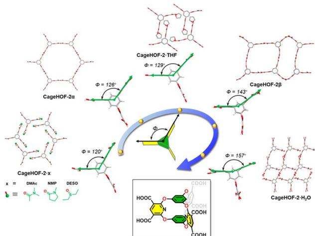
Fig. 12 Schematic illustration of the dihedral angles of the pillar ring changes from 90° to 157° in Cage-6-COOH based structures.<sup>73</sup>
