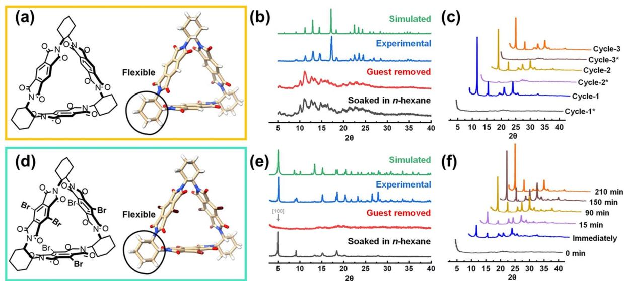
Fig. 10 (a and d) The chemical structures of Tri-PMDI and Tri-PMDI-Br, respectively; (b) PXRD patterns of PMC-Tri-PMDI; (c) PXRD patterns of HOF-Tri-PMDI-Br after removal and re-soaking in *n*-hexane three times; (e) PXRD patterns of HOF-Tri-PMDI-Br; (f) PXRD patterns of HOF-Tri-PMDI-Br soaked in *n*-hexane for different intervals of time.<sup>62</sup>
