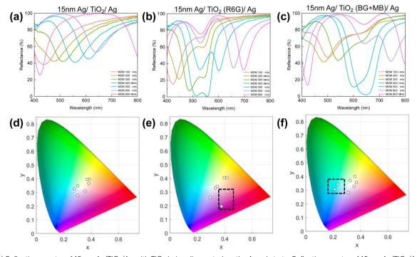
Fig. 26 (a) Reflection spectra of 15 nm Ag/TiO<sub>2</sub>/Ag with TiO<sub>2</sub> being dip-coated on the Ag substrate. Reflection spectra of 15 nm Ag/TiO<sub>2</sub>/Ag with TiO<sub>2</sub> dip-coated from (b) 1 wt% R6G and (c) 1 wt% MB + BG precursor solution. (d)-(f) Resulted coordinates in CIE color space correspond to the spectra in (a)-(c) respectively.
