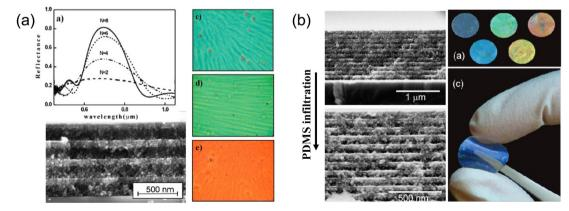
Fig. 13 (a) Optical and SEM image of spin-on alternative SiO<sub>2</sub>/TiO<sub>2</sub> layers of Bragg stacks and their reflection spectra. [Reproduced from ref. 132, with permission from American Chemical Society, Copyright 2008]. (b) PDMS infiltrated inorganic Bragg reflector featuring flexible structural colors. [Reproduced from ref. 133, with permission from American Chemical Society, Copyright 2010].
