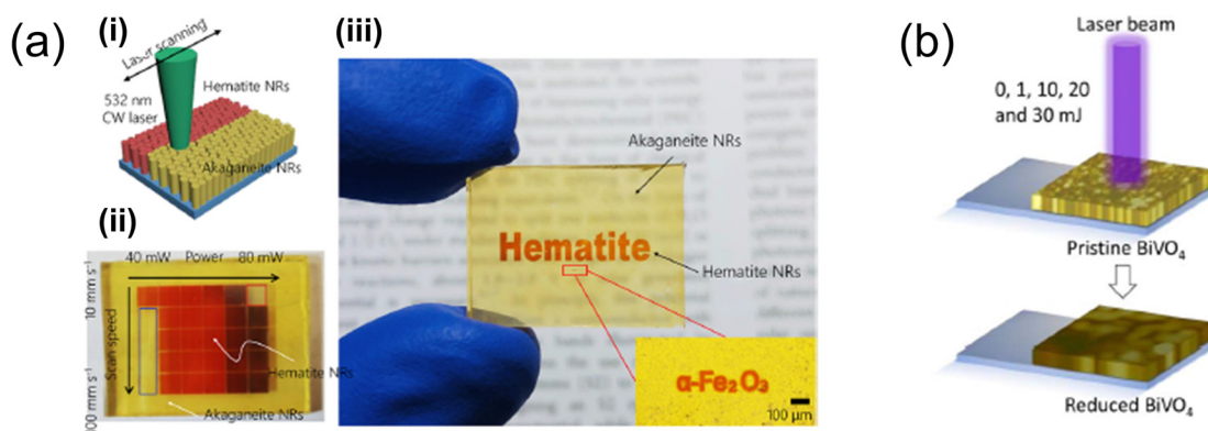
Fig. 7 (a) Illustration depicting (i) the laser-induced selective phase transformation process applied to hematite nanorods (NRs); 88 (ii) combinatorial study of optimal laser power with laser scanning speed for akaganeite NRs on FTO glass substrates; (iii) laser-patterned hematite NRs displaying letters created with the laser scanner. Reproduced with permission from ref. 88, copyright 2020 by American Chemical Society. (b) Schematic showing the laser-based reduction method used for \text{BiVO}_4 photoanodes. 94 Reproduced with permission from ref. 94, copyright 2022 by American Chemical Society.
