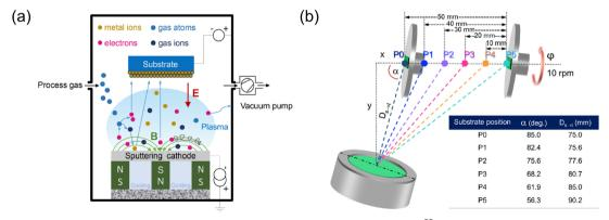
Fig. 3 (a) Schematic representation illustrating the principle of magnetron sputtering technology,<sup>55</sup> adapted with permission from ref. 55, copyright 2020 by Elsevier Ltd and Techna Group S.r.l. (b) Diagram of the magnetron sputtering with glancing angle deposition (MS-GLAD) technique, 56 indicating that the substrate can be adjusted from positions P0 to P5, adapted with permission from ref. 56, copyright 2021 by Elsevier Ltd and Techna Group S.r.l.
