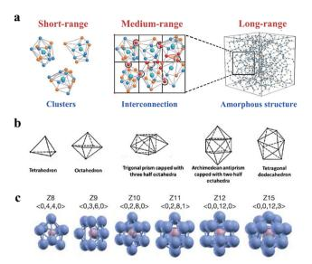
Fig. 2 (a) Schematic illustration of atoms distributed in the short-, medium-, and large-range. Copyright 2022, The Royal Society of Chemistry.<sup>27</sup> (b) Five basic Bernal polyhedrals that describe atomic distribution in the short range. Copyright 1983, American Physical Society. 47 (c) Kasper polyhedron of multi-atomic component of short-range clusters and their symmetry. Copyright 2006, Springer Nature. 48
