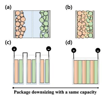
Fig. 1 Schematic illustration of a (a) conventional LIB with liquid electrolyte and (b) ASSB, and batteries with (c) liquid electrolytes and (d) SSEs.
